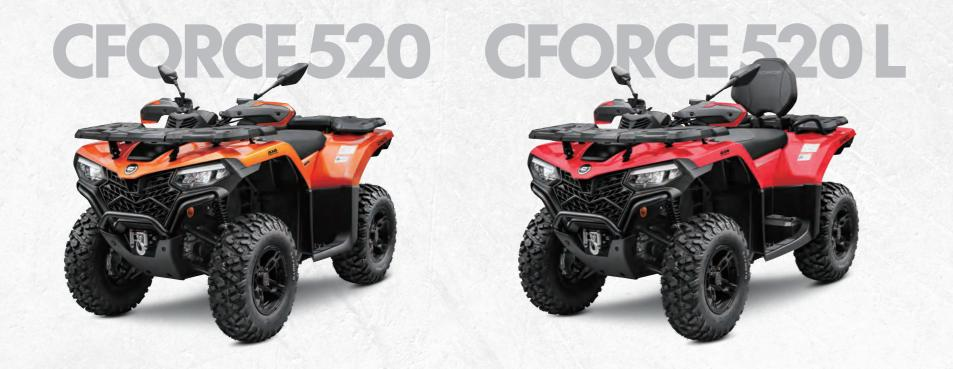
The 495cc engine of the CFORCE 520 adds more power and more possibilities to the agile ATV platform. Fortified with EPS, bigger torque and premium accessories such as RIDEVISION ® LED lights, aluminum alloy wheels, and 25-inch AT tires bring its rugged capability to a new level.
