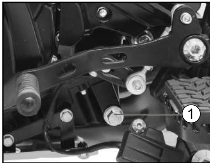
1. Engine oil drain bolt
